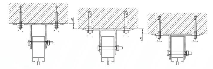
Range of regulation helps avoid problems with the tolerance of wall construction +/-2 cm
